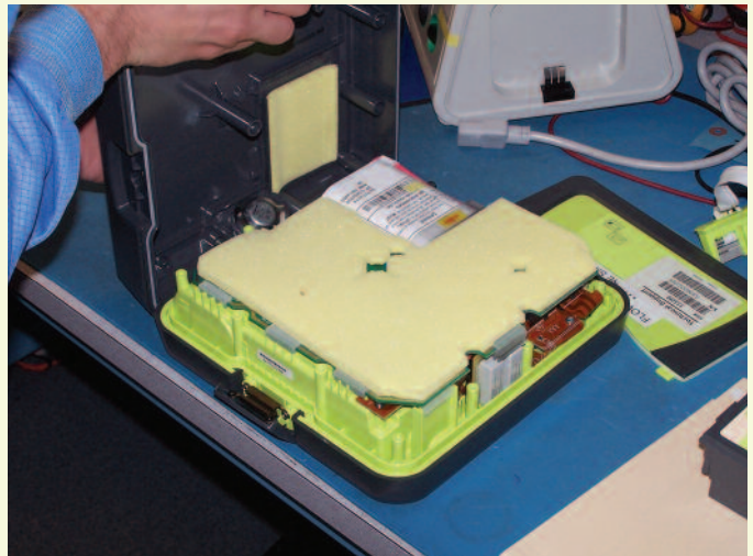
No water damage as the device is opened.
