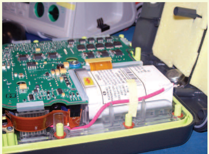
No water damage to the inner electronics.
